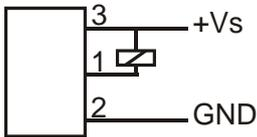
The semiconductor output switches to GND (GROUND = 0 V<sub>DC</sub>) or is highly resistant. The maximum output current is 400 mA.
