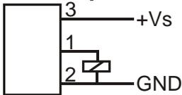
The semiconductor output switches to +24 V<sub>DC</sub> or is highly resistant. The maximum output current is 400 mA. The reference point for the PNP-output is GND (GROUND = 0 V<sub>DC</sub>).
