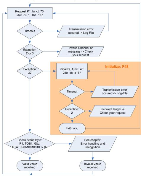
A simple example for reading out a pressure value. Because only one transmitter is connected, the "transparent" address 250 is used.
