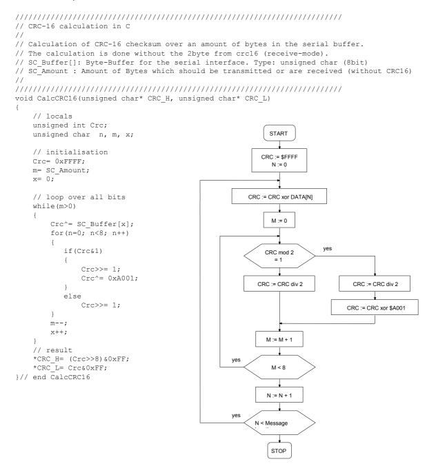
This results in the following calculation for function 48 with device address 250: CRC16\_H= 4, CRC16\_L= 67.
