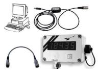
Connect the Castello to the PC using converter cable K104-B (USB) or K107 (RS232). Cable option 5 must be used between the Castello and the converter cable.
