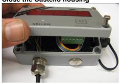
Close the housing and install the four screws.
