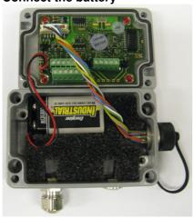
Connect the battery and push it into the battery holder.
