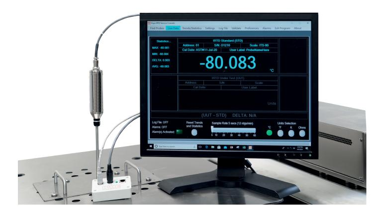
The Kaye IRTD is a high accuracy traceable temperature reference standard used with Kaye Validation systems while calibrating sensors. The broad temperature range from -196°C to 420°C, with an accuracy of +/- 0.025°C, enables it to be used in virtually all temperature validation applications and high-end calibration labs.
