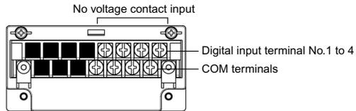
● Alarm relay output (2 points 'c' contact) + Digital input (Non-voltage contact input 4 points)(optional)
