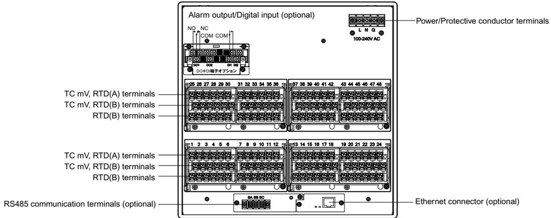
● Alarm relay output (4 points 'c' contact) (optional)
