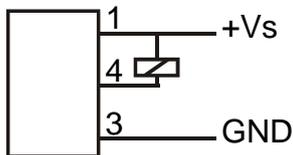
The NPN transistor output either grounds the output pin (GROUND = 0 V<sub>DC</sub>) or is high resistance (open circuit).
