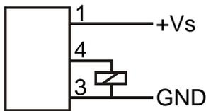
The PNP transistor output either +24 V<sub>DC</sub> or is high resistance (open circuit). The maximum output current is 400 mA.
