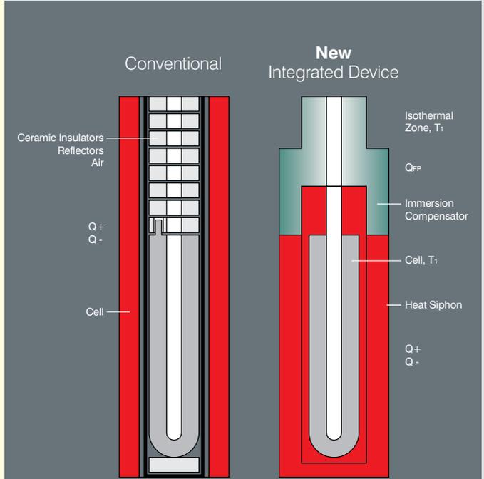
A fixed point cell is not long enough to eliminate heat conduction along the thermometer calibrated in it. Currently, using long furnaces, heat shunts and reflective baffles an attempt is made to reduce these losses.
