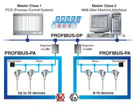
PROFIBUS is a fieldbus network for digital communication over a 2-wire architecture based on the international standard EN 50170. Two levels are used in a PROFIBUS network: the high level PROFIBUS-DP used for process control and the field level PROFIBUS-PA used for field instrumentation.
