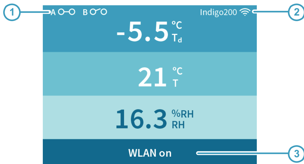
Figure 5 Indigo 201 Display with Relays, Three Parameters and WLAN Notification
