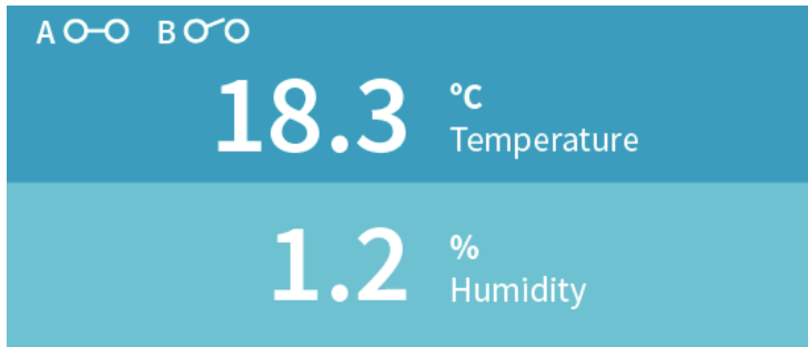
Figure 25 Relay Icons on the Optional Display (Relay A Active, Relay B Not Active)
