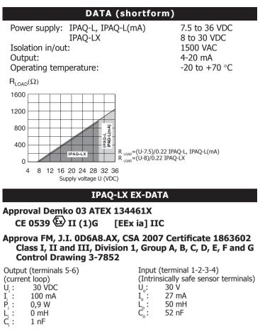
The equipment must be electrically connected (terminal 5 and 6) via a certified isolating interface/zener barrier -and shall be placed outside the hazardous area.
