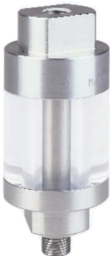
The IDT is an effective barrier for protecting Druck portable pressure calibrators against the ingress of dirt and moisture which may be present in the gaseous pressure media or pneumatic devices under test. Installed directly onto the standard calibrator pressure port, regular use of the IDT 600 will prevent contamination of the calibrator pneumatic system, improving its long term reliability and reducing maintenance costs. In addition it prevents cross contamination of the devices under test.
