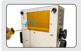
1. Unscrew Two Screws of Battery Cover on the Bottom of the Unit
