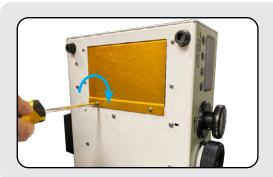
4. Reinstall the Battery Cover by Screwing Back Two Screws
