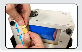
3. Plug the Battery Connector into the Mating Connector
