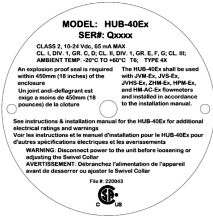
Figure 1: Hazardous Area Certification Tag
