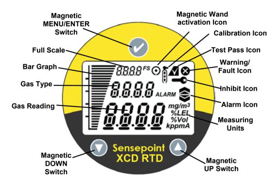
Diagram 2: Sensepoint XCD RTD Display and Magnetic Switches
