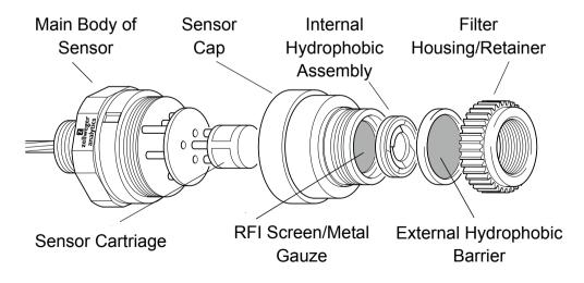
Diagram 16: Sensepoint Toxic Sensor Exploded diagram
