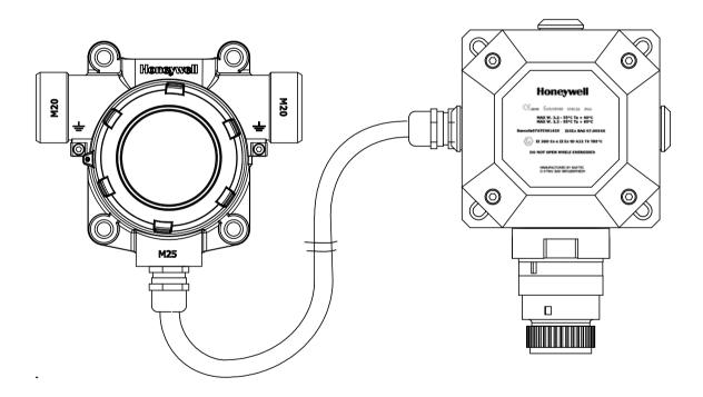
Diagram 7: Remote Sensor Mounting
