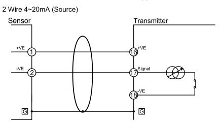
Note: Ensure that the earth from the Sensepoint Toxic Sensor is connected to the Ground/Earth Point.
