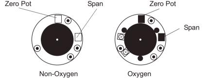
Diagram 15: Sensepoint Toxic Sensor Zero and Span potentiometer
