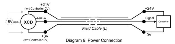
Power consumption of the detector is 5.0W. The current required to drive the detector at the minimum voltage is (I = P / V), 5 / 18 = 278 mA (I detector).
