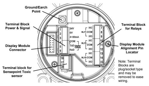
Diagram 8: Sensepoint XCD RTD Terminal module
