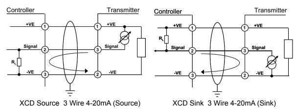
Note: Terminate cable screen at transmitter or controller, not both.
