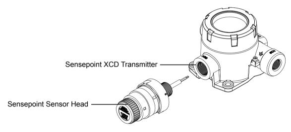
Diagram 6: Installing the Sensor
