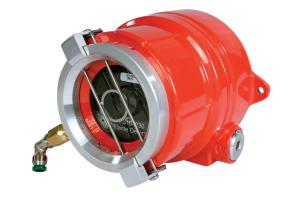
A high-speed microprocessor based fire detection and process control system specially designed for liquid and powder coating applications, the FS10 System quickly detects the presence of a flame, reacts by initiating a shutdown of the electrostatic finishing process in a matter of milliseconds and effectively interrupts the fire before residues and wet paint films can ignite.
