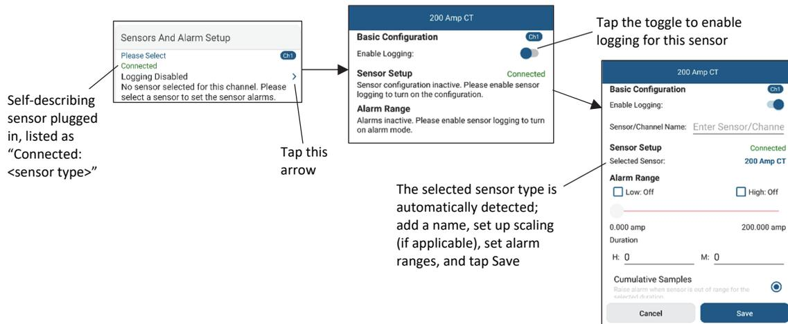
**Sensors & Alarm Setup Setting**
