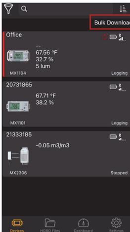
2. The screen changes to Bulk Download mode. This changes the way the screen behaves when you tap on a logger tile. Tap on a tile to select it for Bulk Download. You can select up to 20 loggers. Text at the bottom of the page updates to indicate how many loggers are selected.
