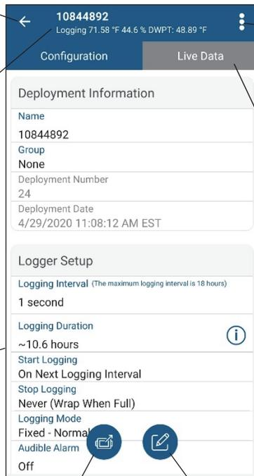
On iPhones®, iPads®, or Android devices, tap to view more details about the logger and access logger password, stop logging, and other features (see *Logger Details and Actions*). **Note:** These features are all on the main screen in the Windows version.
