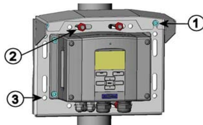
Figure 15 Mounting the Rain Shield with the Installation Kit
