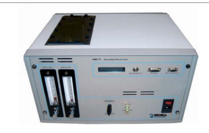
A low-cost, easy to use, fully integrated system for the calibration of dew-point and relative humidity sensors from 2 to 90% relative humidity, -30 to  $+20^{\circ}$ Cdp (-22 to  $+68^{\circ}$ Fdp).
