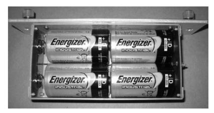
Replace the battery box and tighten thumbscrews.
