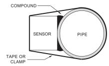
Over time temporary coupling compounds (e.g. Petroleum Gel) may gradually sag away from the sensor resulting in reduced signal strength and finally complete loss of signal. Warm temperatures, moisture and vibration will accelerate this process. Dow Corning Silicone Compound #4 as supplied with the PDFM 5.1 (and available from Greyline Instruments) is recommended for semi-permanent installations.
