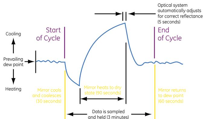
The PACER cycle works very well, but eventually manual cleaning may be required. All of GE's chilled mirrors are accessible for manual cleaning. Cleaning is a simple process consisting of wiping the mirror with a cotton swab wetted with cleaning solution or distilled water.
