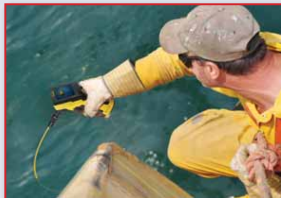
The entire SeaScope™ system - including the grip, monitor and probe - is guaranteed watertight to a depth of 1 meter
