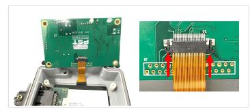
Figure 3: Location and insertion of LCD ribbon cable
