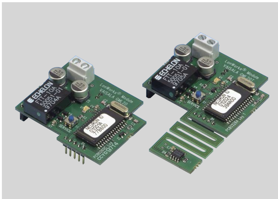
GML20 (left) and GML20T modules enable digital communication between the Vaisala CARBOCAP® Carbon Dioxide Transmitter Series GM20 and a LonWorks® network.
