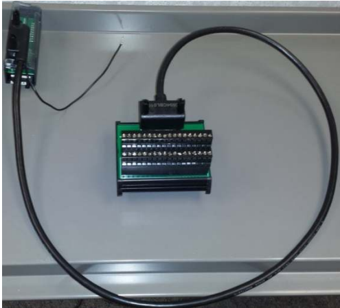
Figure 447: High-Density Compact Remote Terminal Base IC694RTB032 Usage
