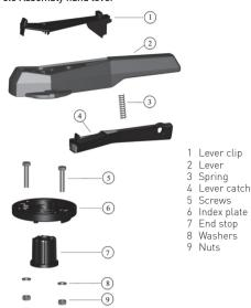
Hand lever assembled by closed disc. By the indexa-tion of the shaft and the end stop a clear assembly is
