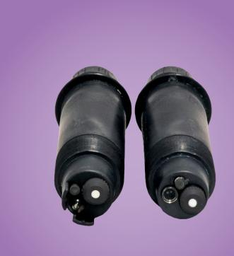
Process electrodes built with superior glass formulation, 3-electrode differential design and protected reference electrode housed in a glass half-cell to withstand extreme pH conditions, elevated temperatures and poisoning ions. These sensors are suitable for continuous monitoring of pH and ORP in a wide range of heavy duty applications.
