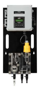
The Signet 4632 Chlorine Dioxide Analyzer System is an integrated all-in-one system designed to measure Chlorine dioxide residual up to 2 ppm/mg/l.
