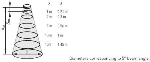
**Minimum measuring distance (X\_m)** is determined by the design of the unit within which the measurement is not possible (Dead Zone) its value is according with P05. Since measurement is impossible within this range material should not get into this zone
