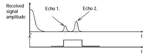
Some applications involve multiple (target + disturbing) echoes even within the measuring window. Basic echo selection will be done by the Quest + software automatically. This parameter influences the echo selection only within the measuring window.
