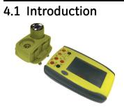
This section gives examples of how to connect and use the instrument to measure pressure with the module carrier (MC 620-IS) and the applicable pressure modules (PM 620-IS).
