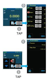
If necessary, change the *Process* for the CH1 and/or CH2 measure functions: item
