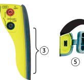
**3. •**← : USB mini Type B connector for communication with a computer.
