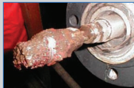
► Glycol carry-over and dirt on this transducer was not enough to stop GE's robust transducer technology in this pipeline gas application
