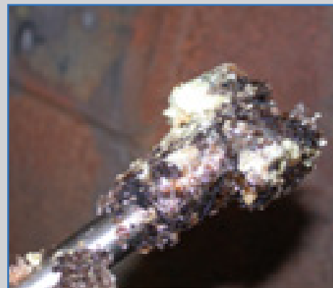
► Despite this significant amine crystal build up, these transducers continued to operate reliably
