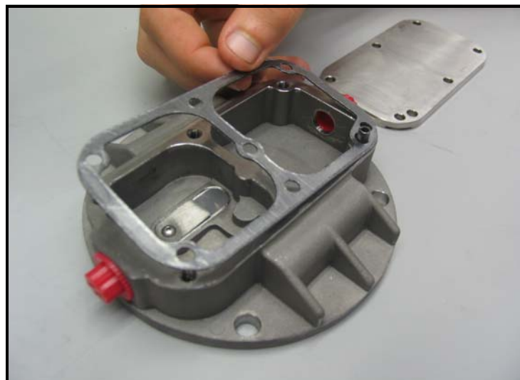
Figure 76: Installing the New Valve Cover Gasket
