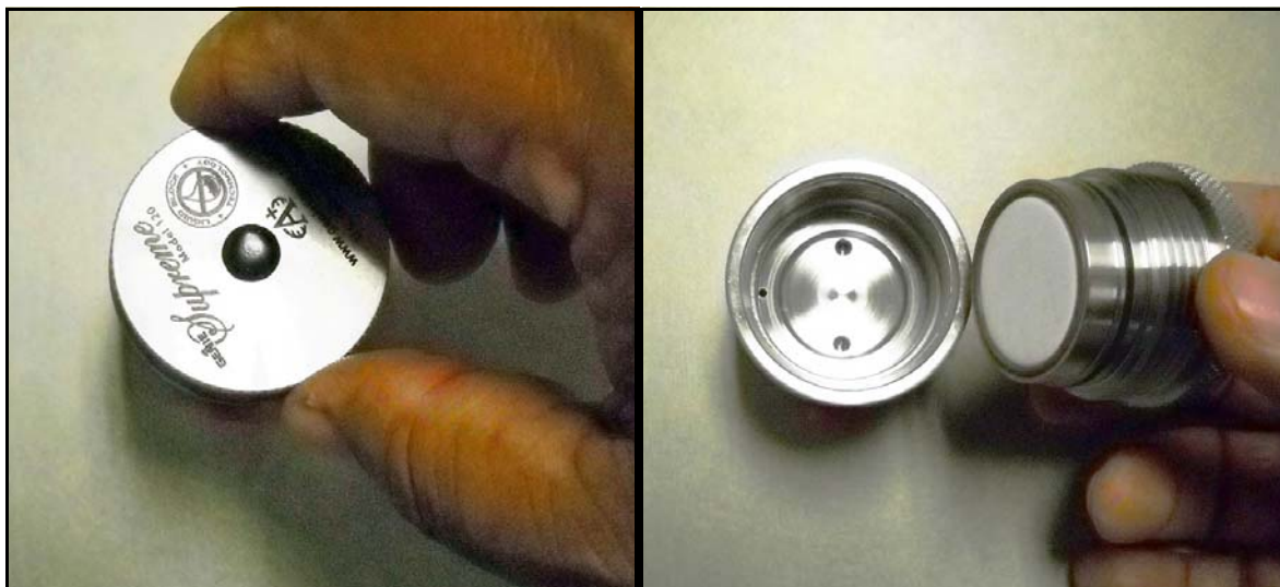
Figure 66: Removing the Filter Cap
