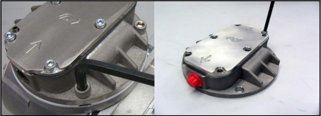
Figure 73: Removing the Head Section and Socket Head
