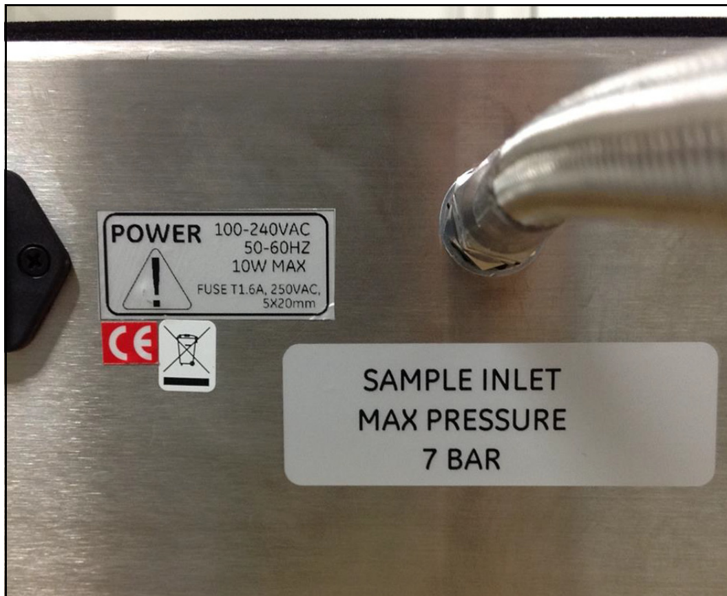
Figure 7: Power, CE and Inlet Labels
