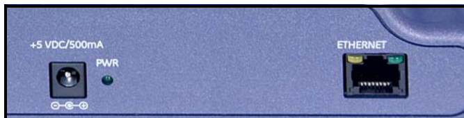
Figure 36: Base Station Connections
