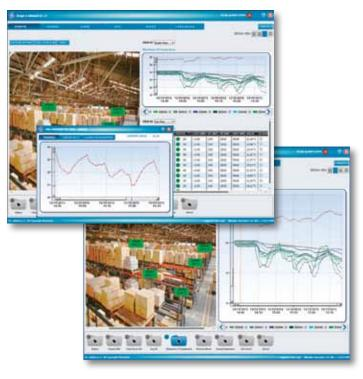
Historical graphing provides the user with the ability to pre-select a group of sensors and create a template for the group and trend. Users may view up to 24 hours of data of up to 1440 samples per single tag input. The user has the ability to export the data from the graph to a bitmap file or printer for further analysis.
