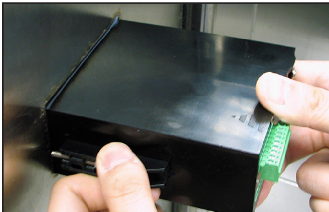
Figure 13: Locking the Mounting Brackets in Place
