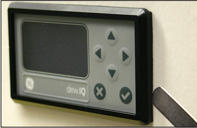
Figure 15: Checking the Gasket Compression
