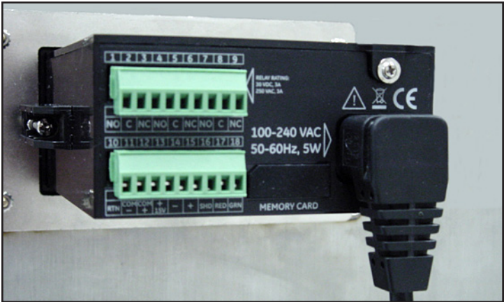
Figure 32: The AC Power Cable Installed
