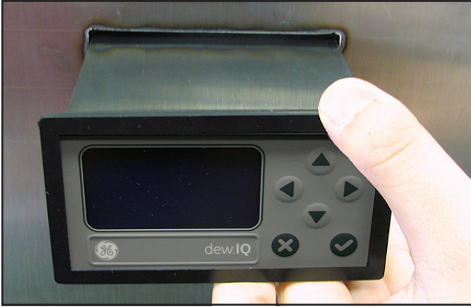
Figure 11: Sliding the dew.IQ into the Panel Cutout
