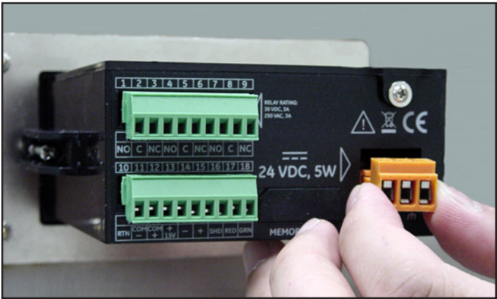
Figure 33: Removing the DC Power Connector
