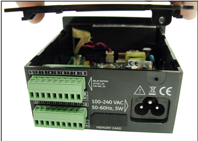
Figure 7: Removing the Cover
