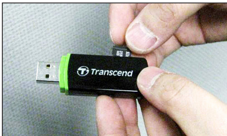
Figure 52: Plugging the MicroSD Card into a Card Reader
