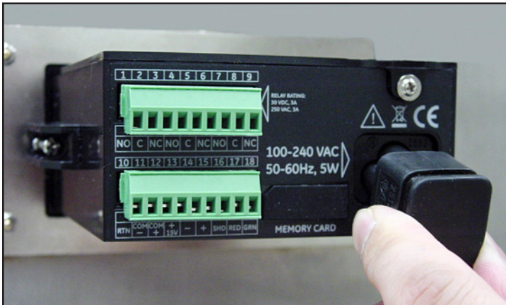
Figure 31: Inserting the AC Power Cable
