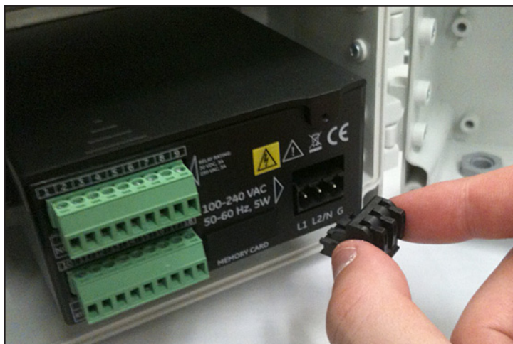
Figure 35: Removing the AC Power Connector
