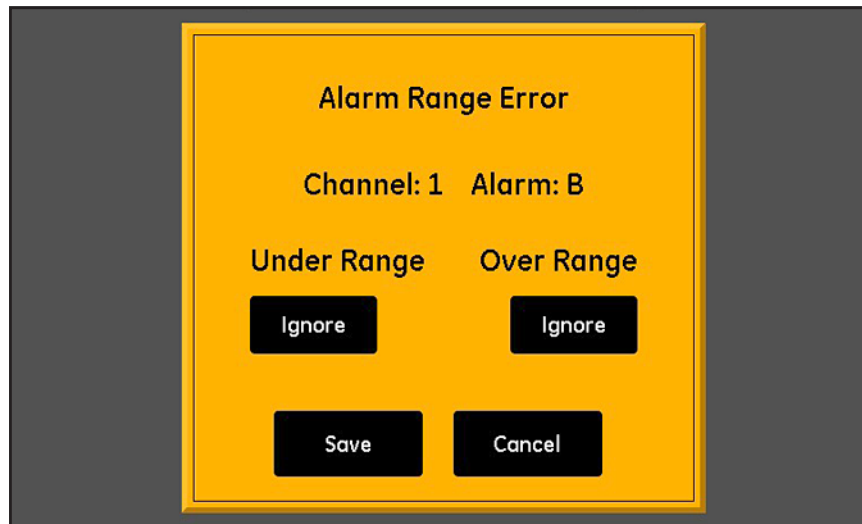
Figure 49: Range Error Setup Screen - Alarm Response
