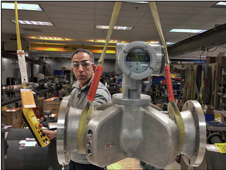
Figure 5: Lifting the PanaFlow Z3 System
