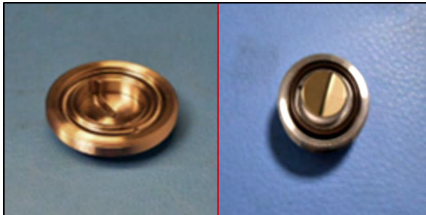
Figure 91: Replacing Cleaned Mirror into End Cap Assembly
