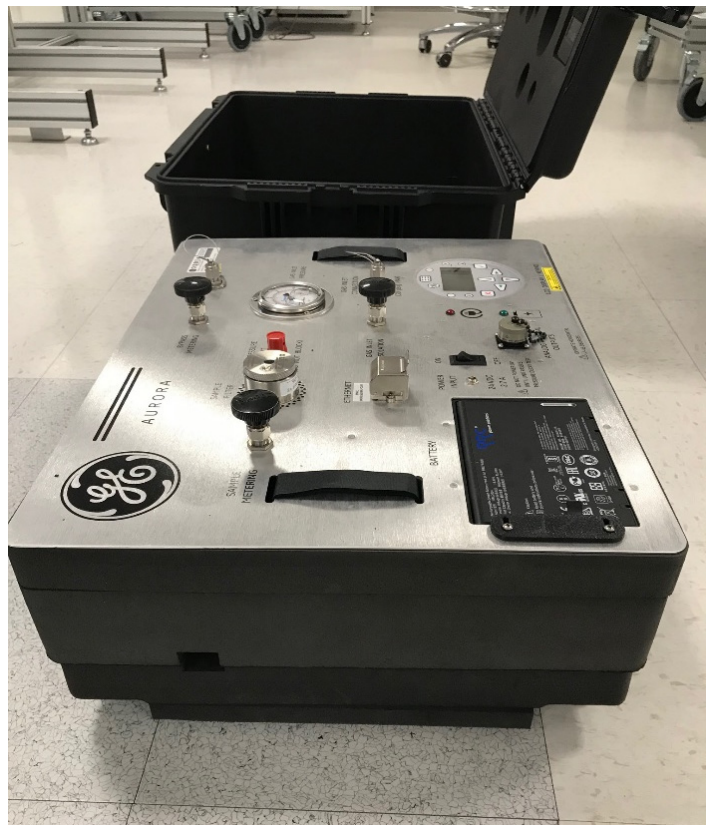
Figure 52: Extraction of Inner Foam Assembly from TransPort Pelican Case for Access to Absorption Cell End Mirror
