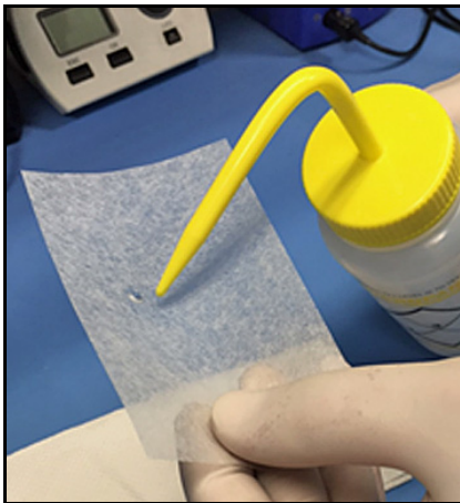
Figure 56: Applying Acetone to Lens Tissue
