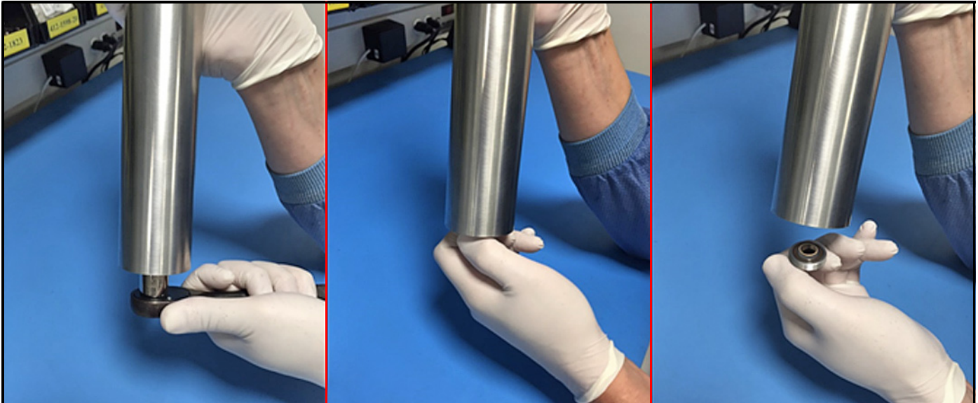
Figure 54: Removing Mirror End Cap Assembly from the Absorption Cell
