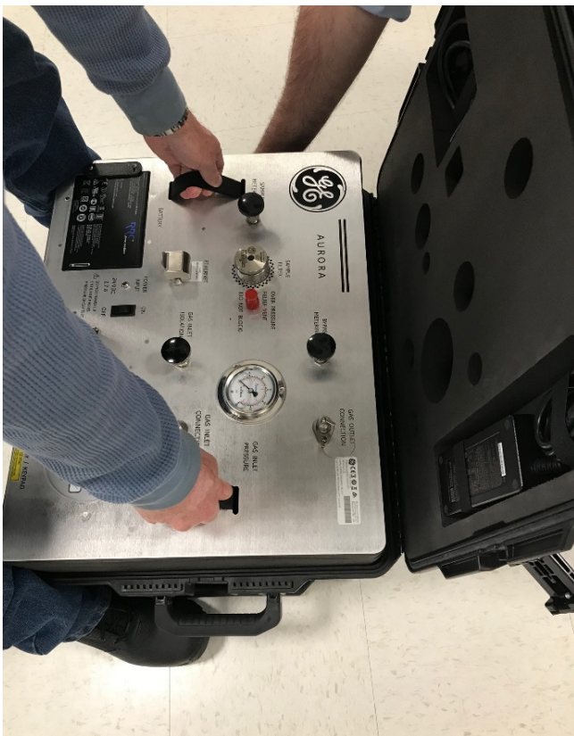
Figure 52: Extraction of Inner Foam Assembly from TransPort Pelican Case for Access to Absorption Cell End Mirror
