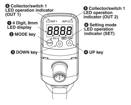
Pressing the MODE key for 3 seconds displays "\_\_\_\_"To return to measurement mode, the " display will flash when 3 seconds have passed.
