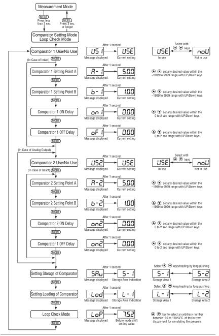
In "Comparator setting mode," user can change settings on the comparator outputs provided by the unit. (Two comparator outputs or one for analog output unit are provided). The available selections of this mode varies based on the selections made in Function setting mode and comparator output type selection. For the unit provided with two comparator outputs, settings of each output can be done independently with the exception of the operation mode.
