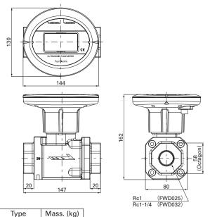
Wafer connection type <Nominal diameter: 40 to 80mm>
