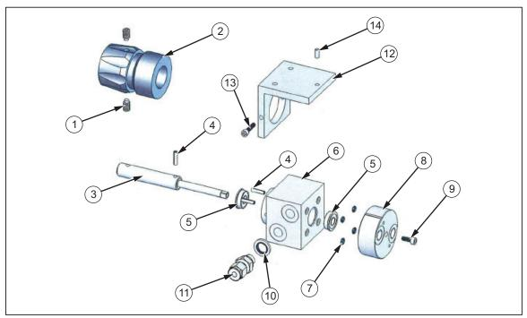
Figure 5-6. System Selector Valve
