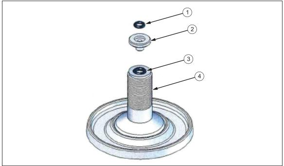
Figure 2-6. Test Port Insert
