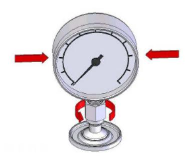
Figure 2-5. Tighten Gauge
