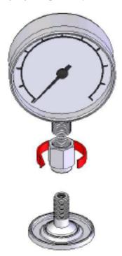
Figure 2-1. Screw on Gauge Adapter
