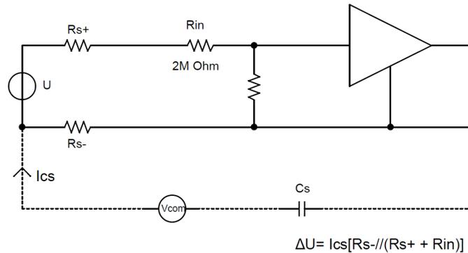
**Appendix Figure 3. Effects of Leakage Current on Voltage Measurement**
