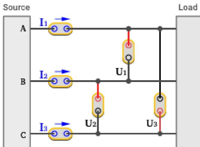
**Figure 10. 3P3W3M Wiring**
