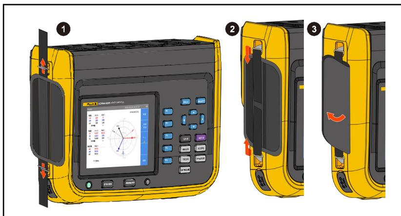
**Figure 3. Install the hand strap**
