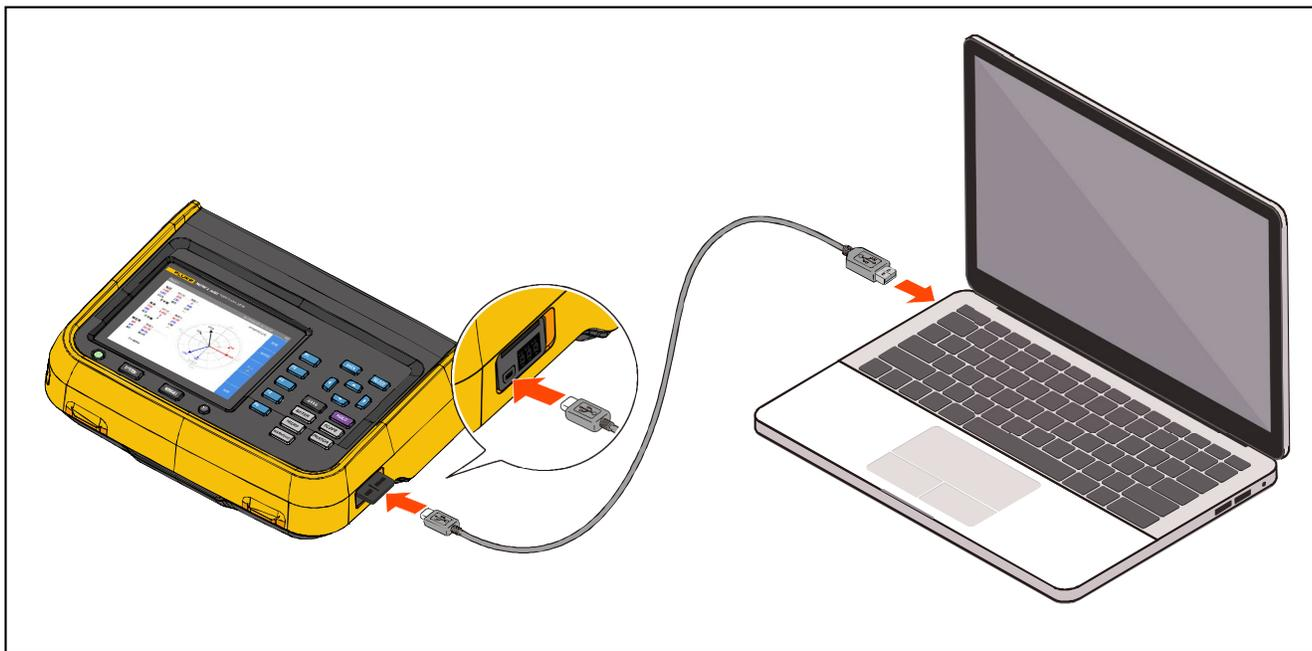
**Figure 22. Connect the Computer**
