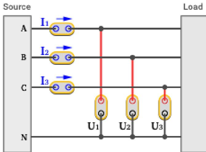
Figure 9. 3P4W3M Wiring
