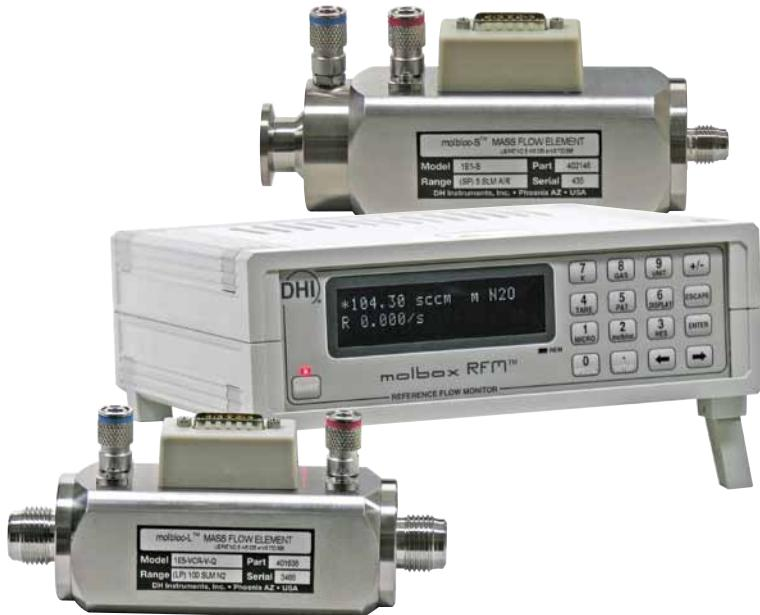
molbox RFM is a support unit for making mass flow measurements using molbloc-L laminar and molbloc-S sonic flow elements.
