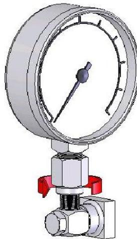
**Figure 2. Connect Assembly to Test Port**
