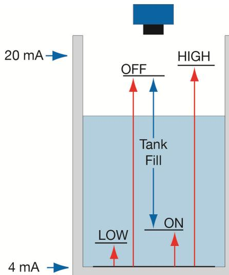
**Note:** All relay settings are referenced from the Empty or 4mA setting of the tank.
