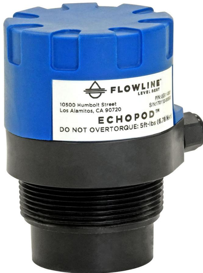
An ultrasonic sound wave is pulsed from the base of the transducer. The sound wave reflects against the process medium below it. The sound wave energy is returned to the transducer. The microprocessor based electronics measures the time of flight between the sound pulse generation and its receipt. This translates into the distance or range between the transducer and process media below.
