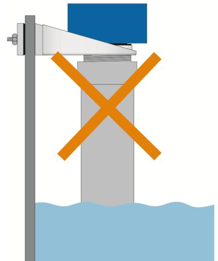
**Note:** The Side Mount Bracket (LM50 series) is not designed for use with stand pipes or as a method to secure stand pipes. There are too few threads to properly hold the sensor and the stand pipe.
