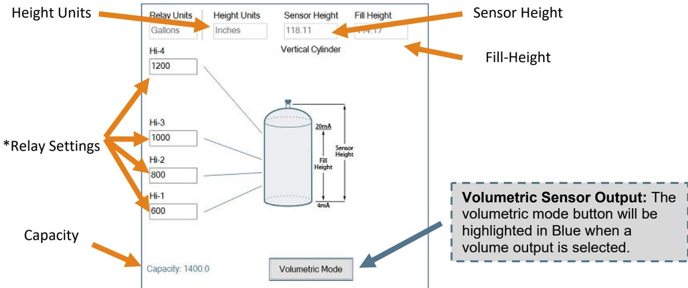
\* Relay settings are based upon the configurations selected under the Config pull-down menus.
