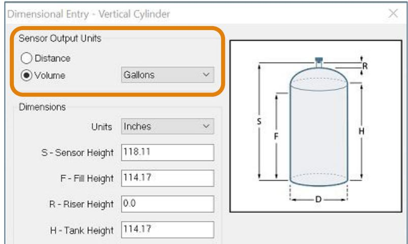
**Volume – Tank Capacity (Vertical Cylinder Example):** After entering the dimensions, press the Capacity button to show the Calculated Capacity of the tank. If the Calculated Capacity is slightly different than the expected capacity, click on the Adjust Capacity box and enter the expected capacity of the tank. If the Adjusted Capacity is more than 10% of the Calculated Capacity, recheck the dimensions information entered above.
