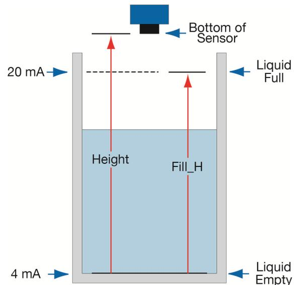
3. **Relay Set Points** – Distance from the bottom of the tank to the level of liquid where each relay activates.
