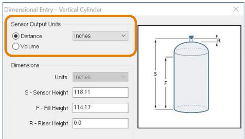
**Volume – Sensor Output Units (Vertical Cylinder Example):**
