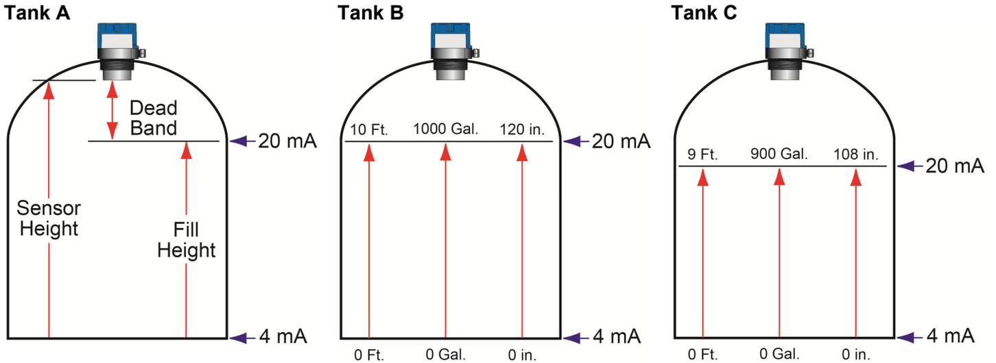
In the **Tank A** example, the Sensor Height sets the 4mA to the bottom of the tank. Fill-Height sets the 20mA to the top of the straight side of the tank.
