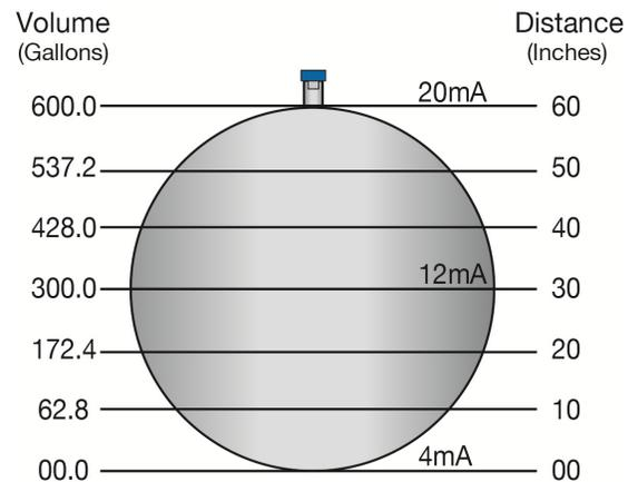
**Note:** In the above illustration, 1" of liquid does not equal 10 gallons. The 10" at the bottom represents a rise of 62.8 gallons. As a change between 10" and 20" represents an increase of 109.6 gallons (i.e. 172.4 gallons – 62.8 gallons).
