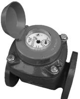
FloCat-W Turbine Meters are horizontal Woltman type water meters designed for accurate, economical reading of medium-to-high flow rates with minimal pressure loss. Rugged cast iron meter bodies are epoxy-coated inside and outside. The turbine drives a vertical impeller in direct proportion to the water flow. The impeller is magnetically coupled to the register, which contains a removable dry contact reed switch pulse output and does not require power.
