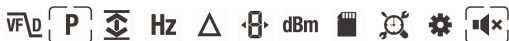
Figure 5.2 Mode icons (AC voltage measurements): Peak mode and Silent mode are enabled
