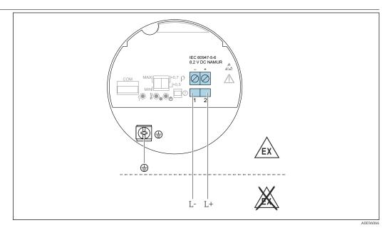
■ 13 2-wire NAMUR  $\geq$  2.2 mA/ $\leq$  1.0 mA, electronic insert FEL68
