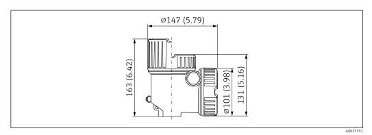
■ 36 Dual compartment, L-shaped; aluminum, coated; with Ex d/XP approval also; Product Configurator: order code for "Housing; material", option M. Unit of measurement mm (in)
