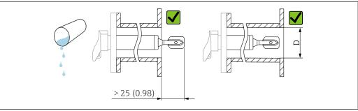
**2**2 **2**2 Installation example for low-viscosity liquids. Unit of measurement mm (in)
