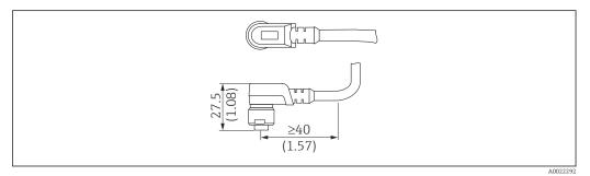
■ 50 Plug-in jack M12 IP67. Unit of measurement mm (in)
