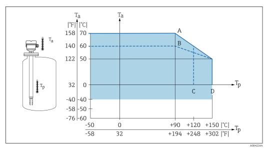
$\blacksquare$  30 Permitted ambient temperature  $T_a$  at the housing as a function of the process temperature  $T_p$  in the vessel:
