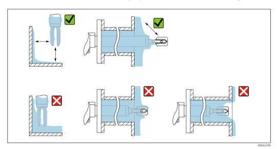
$\blacksquare$  24 Installation examples for a highly viscous process medium
