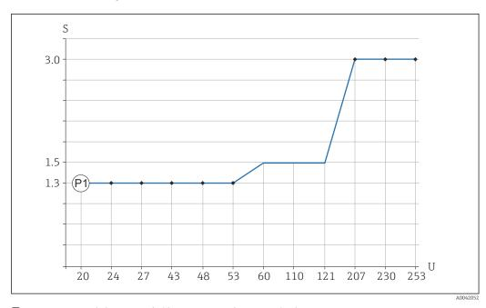
$\blacksquare$  4 Recommended minimum holding power/rated power for load
