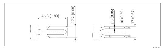
$\blacksquare$  40 Tuning fork with enamel coating. Unit of measurement mm (in)
