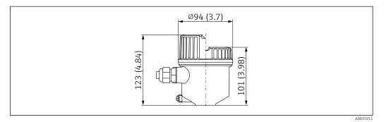
Single compartment; plastic; Product Configurator: order code for "Housing; material", option A. Unit of measurement mm (in)
