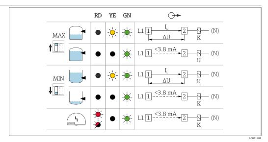
$\blacksquare$  3 Behavior of switch output and signaling, electronic insert FEL61
