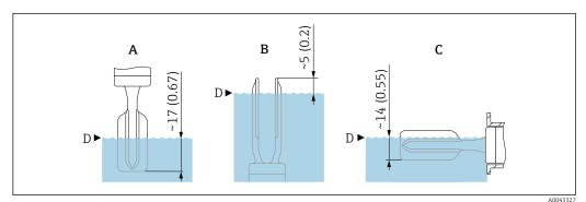
■ 18 Typical switch points, enamel-coated tuning fork. Unit of measurement mm (in)
