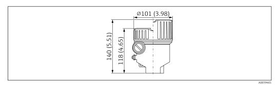
■ 33 Single compartment; aluminum, coated; with Ex d/XP approval; Product Configurator: order code for "Housing; material", option B. Unit of measurement mm (in)
