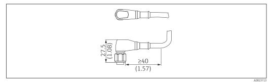
49 Plug-in jack M12 IP69. Unit of measurement mm (in)
