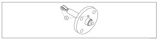
■ 26 Marking on flange to align the tuning fork
