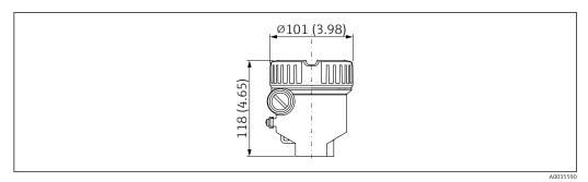
■ 35 Single compartment 316L, cast; with Ex d/XP approval also; Product Configurator: order code for "Housing; material", option C. Unit of measurement mm (in)
