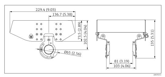
$\blacksquare$  47 Weather protection cover for dual-compartment housing, aluminum. Unit of measurement mm (in)
