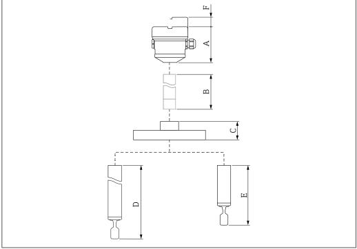
᠍ 31 Components for calculating the device height
