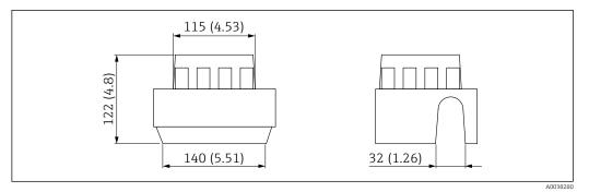
$\blacksquare$  48 Protective cover for single compartment housing, aluminum or 316L. Unit of measurement mm (in)
