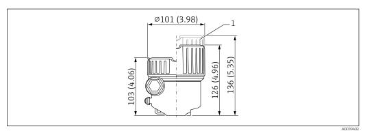
■ 34 Single compartment; aluminum, coated; Product Configurator: order code for "Housing; material", option B. Unit of measurement mm (in)
