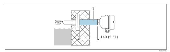
**■** 37 Temperature spacer, pressure-tight feedthrough (1). Unit of measurement mm (in)
