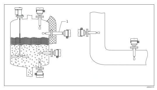
Examples of installation in a vessel, pipe or tank
