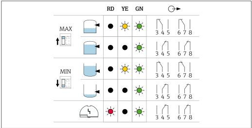
Behavior of switch output and signaling, electronic insert FEL64 DC
